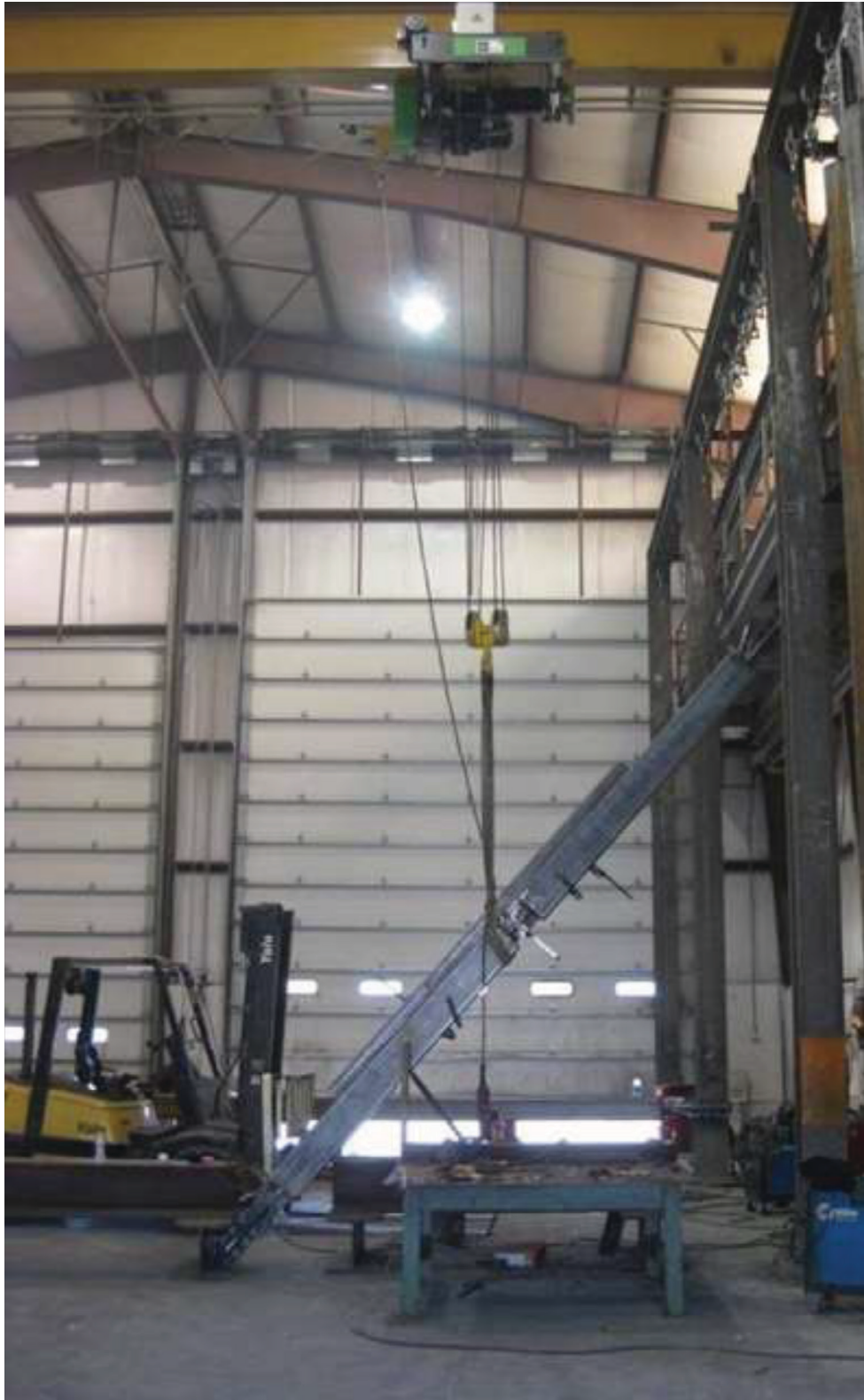
Fig. 11. Prototype spliced in inclined position.
