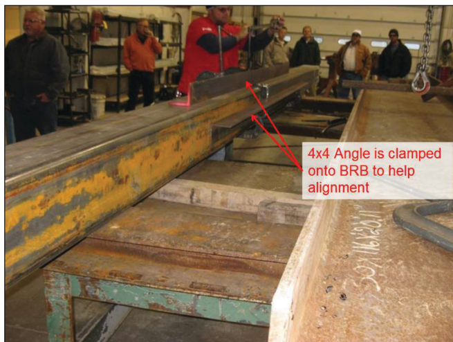
Fig. 9. Alignment aid for casing.
