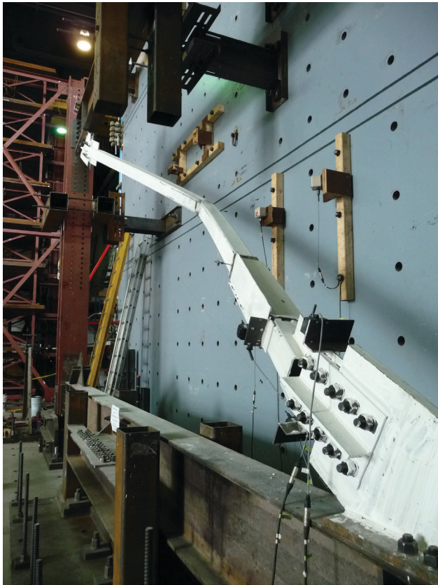
Fig. 10. Ductile tension fuses for HSS braces: (a) fabrication details; (b) full-scale testing in a re-usable test vertical frame; (c) typical hysteretic responses with and without fuses (illustrations courtesy of Professor Robert Tremblay).
