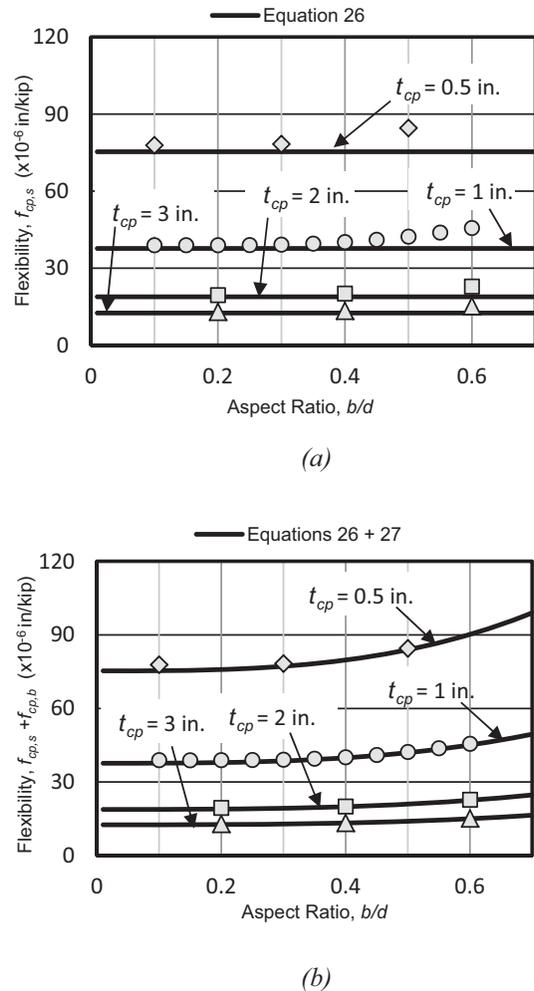
Fig. 20. Correlation of continuity plate flexibility: (a) shear component only; (b) flexural and shear components.
