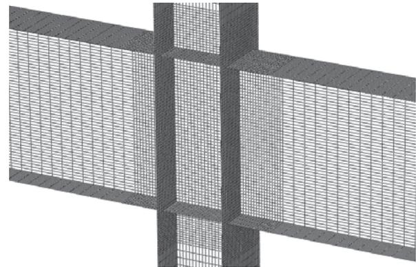
Fig. 9. Finite element mesh in the connection region.
