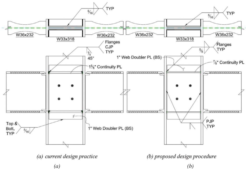
Fig. 24. Comparison of continuity plate and weld design of an RBS moment connection with a deep column:
