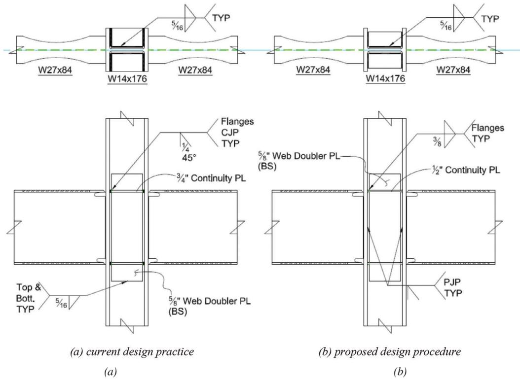
Fig. 23. Comparison of continuity plate and weld design of an RBS moment connection with a W14 column:
