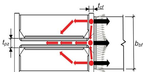
Fig. 15. Flow of beam flange force to column.
