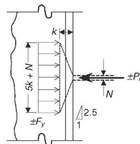
Fig. 5. Local force transfer for WLY limit state (Carter, 1999).
