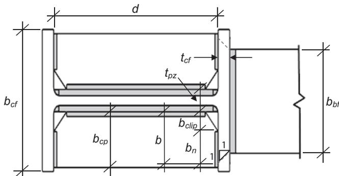
Fig. 21. Net bearing width of continuity plate.
