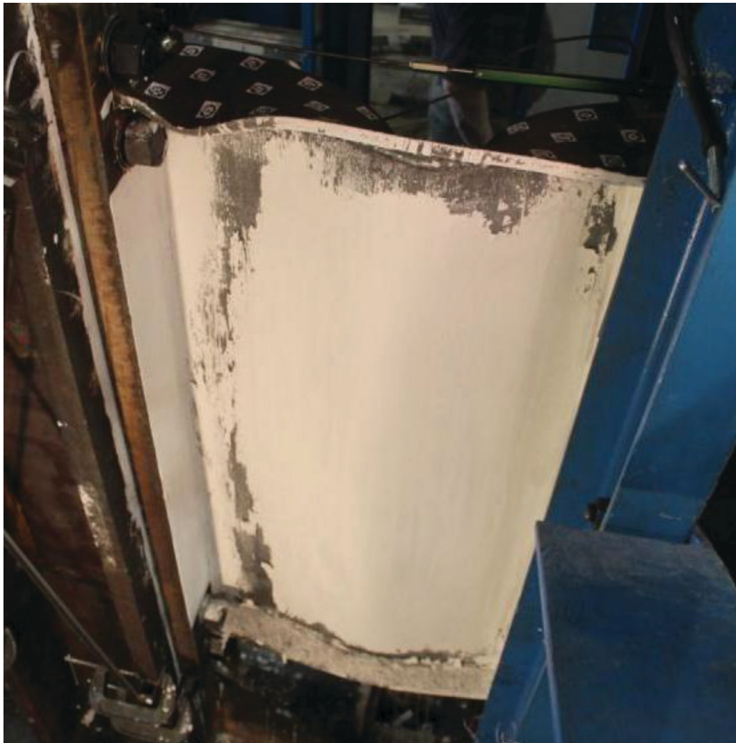
Fig. 7. Full-scale test of 48-in. slender web beam with end-plate moment connection (photograph courtesy of Professor Matthew Eatherton).
