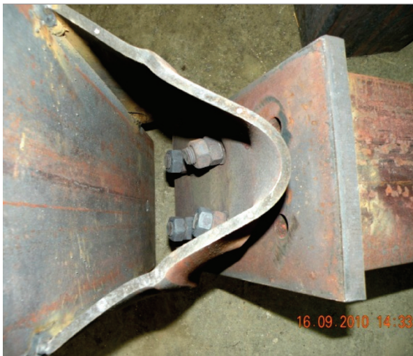
Fig. 3. Typical failure mode of a reverse-channel connection (photograph courtesy of Professor Ian Burgess).
