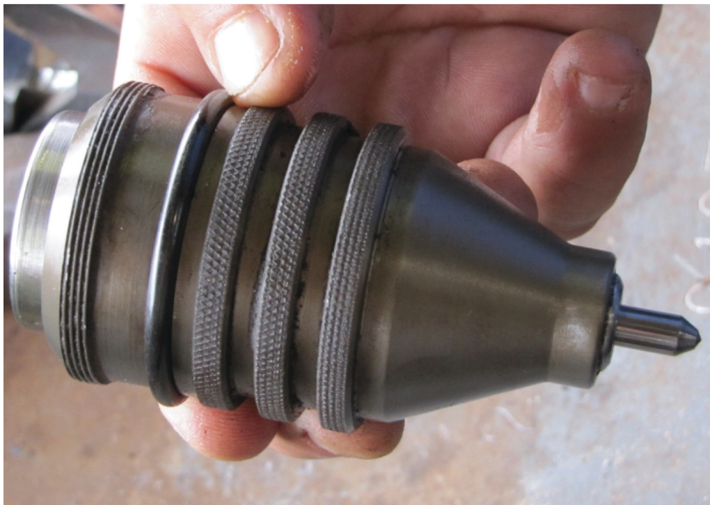
Fig. 5. Stylus used to mark specimen.
