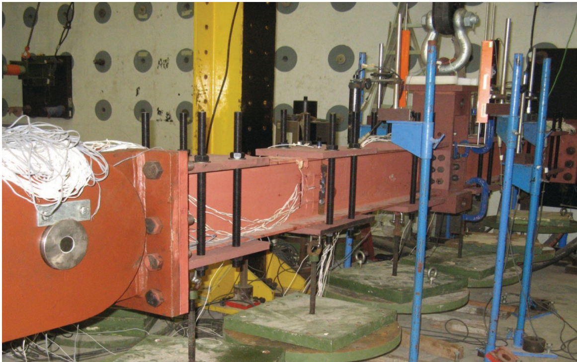
Fig. 11. Details of test setup for collapse after column removal. (Photograph courtesy of Professors T.-C. Fung and K.-H. Tan)
