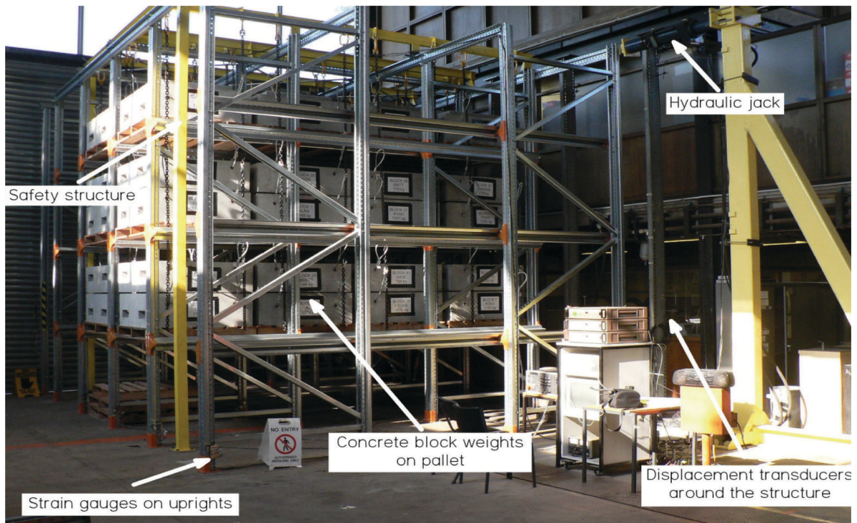
Fig. 5. Full-scale rack test. (Figure courtesy of Professor Kim Rasmussen)
