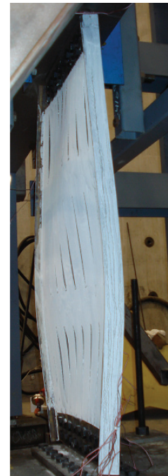
Fig. 5. Global lateral-torsional buckling of an SSP.
